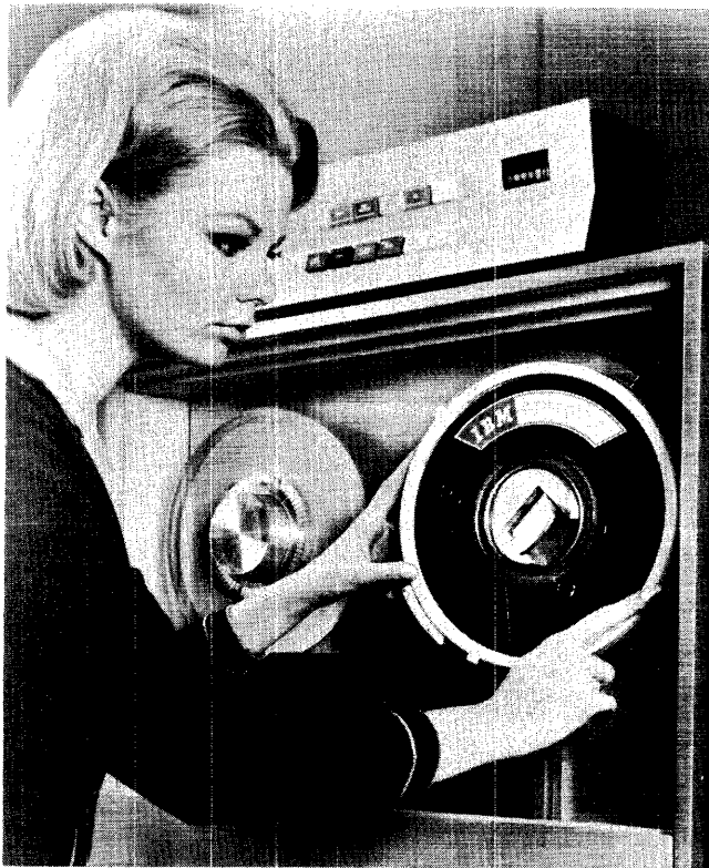
Figure 7-30. IBM 2420 Magnetic Tape Unit Model 7 with Wraparound Cartridge
