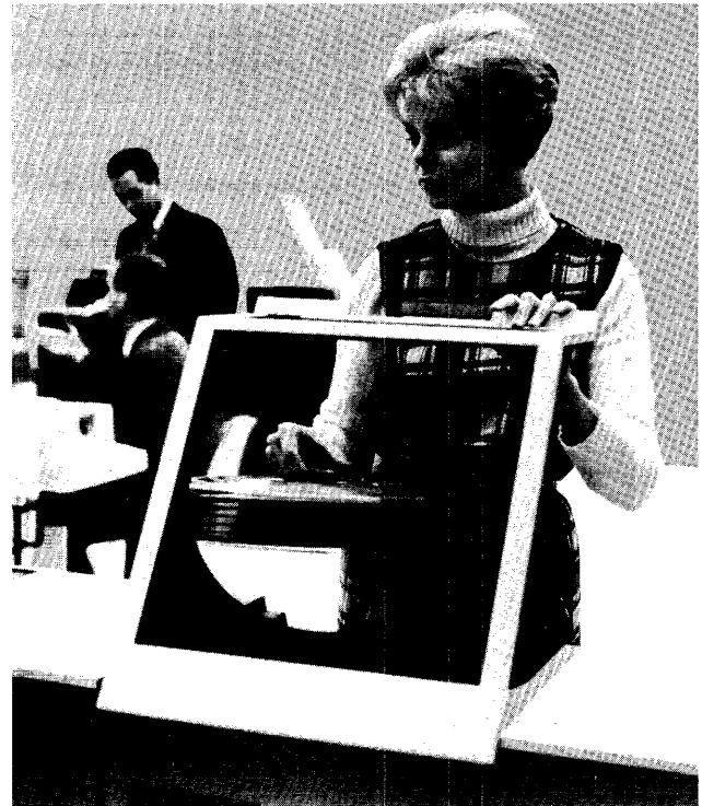
Figure 7-5. IBM 1316 Disk Pack Being Placed in an IBM 2311 Disk Storage Drive
