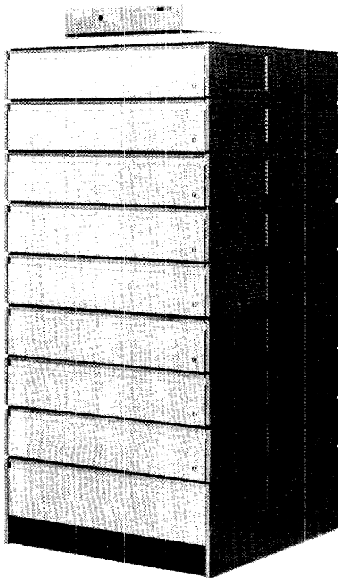
Figure 8-6. IBM 2711 Line Adapter Unit (with Maximum Number of Line Adapter Modules)
